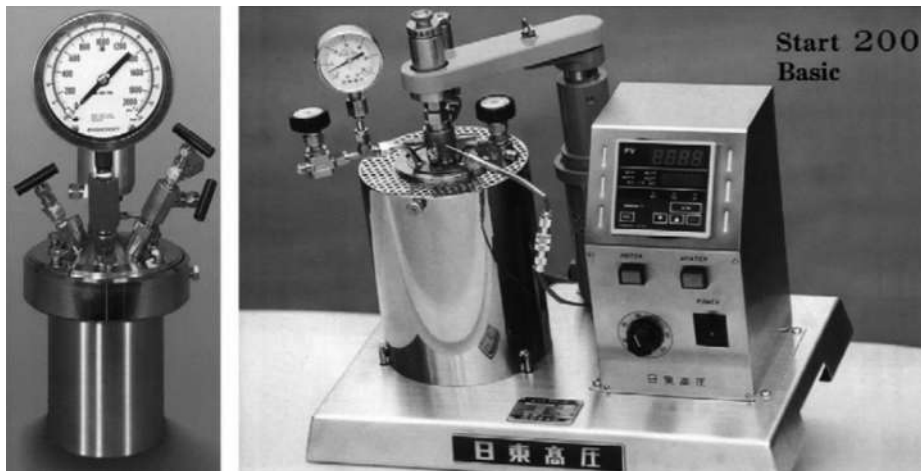
Figure 11. Commercially available, magnetically stirred stainless steel pressure vessel configured with pressure control and an external pump to control the gas flow (37). Reproduced with permission from ref (37). Copyright 2007 Elsevier Ltd.
