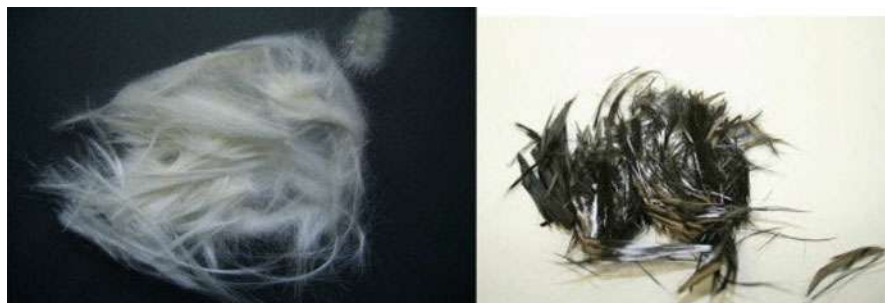
Fig. 9 Recovered glass fiber (left) and carbon fiber (right) from treatment in BZA (Goto 2009)
