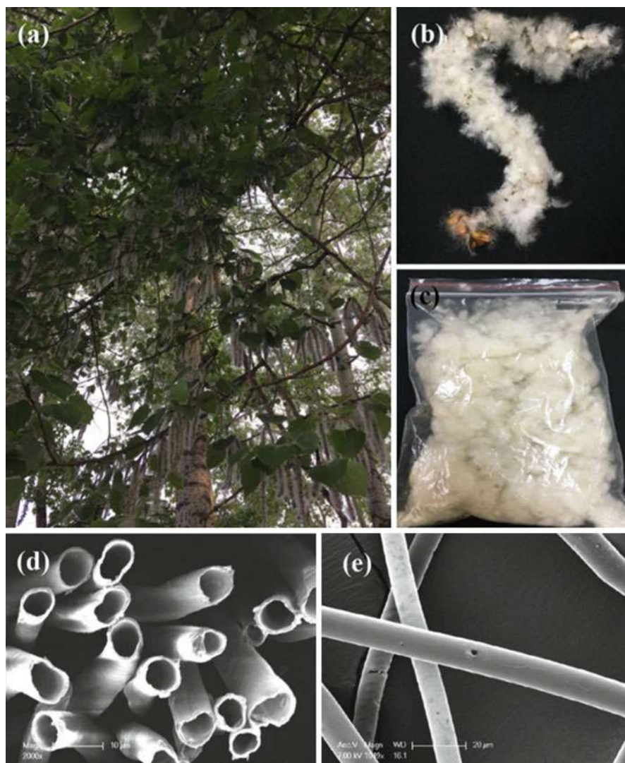
Fig. 7 The Photos from, (a) the poplar tree, (b and c) poplar catkin fibers, (e and f) SEM image of poplar fibers. (Reprinted from Zhang et al. (2018) as open access source of Springer Nature)
