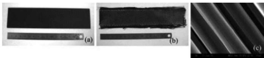
Fig. 11 Appearance of recovered carbon fiber from CFRP at 270 °C, 8 MPa and 90 min: (a) CFRP before decomposition, (b) recovered carbon fiber after decomposition, and (c) SEM photo of recovered carbon fiber with 3000 magnification (Okajima et al. 2014)
