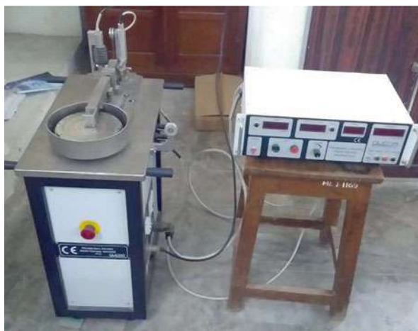
Fig. 14 Pin-on-disc wear test
