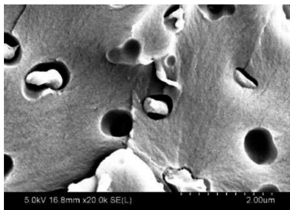
Fig. 6 SEM image of fractured samples at 5 w% loading (Al-Assafi et al. 2016)
