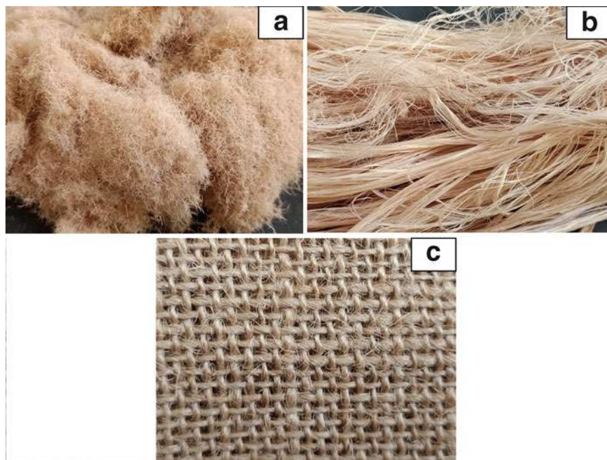
Fig. 1 Fiber types: (a) random chopped fiber, (b) long fiber (c), plain weave woven fiber
