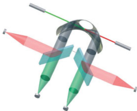
Figure 7.14 The scheme of the Dual Wavelength Optical Particle Spectrometer (DWOPS).
