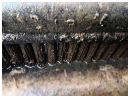
Figure 4. Fouled MBR membrane.
