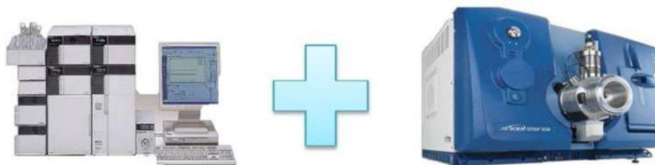
Figure 3. LC-MS method for detection of preservatives in cosmetics.
