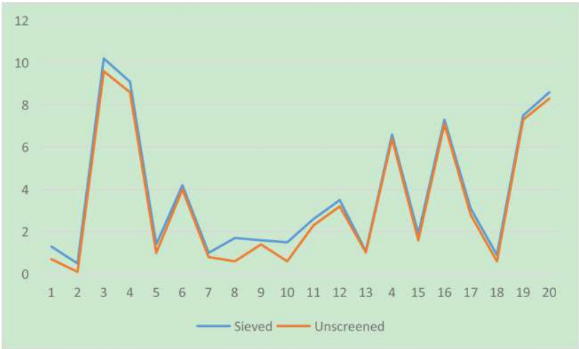
Figure 2. Pb content of ceramic tiles at different powder particle sizes.
