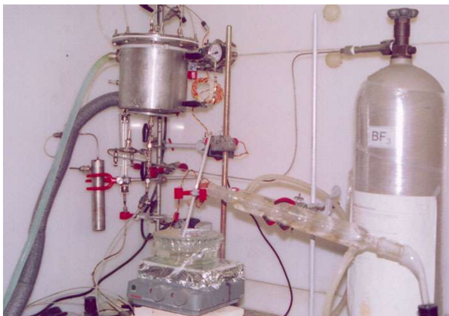
Figure 25.2 Polymerization system equipped with a stainless steel reactor.
