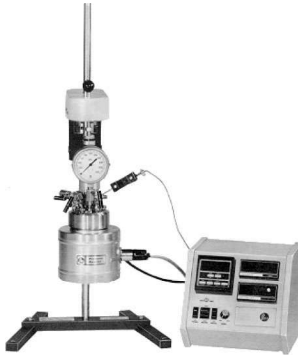
Figure 25.11 Schematic representation of the reactor used in catalytic tests, Parr autoclave (with permission).
