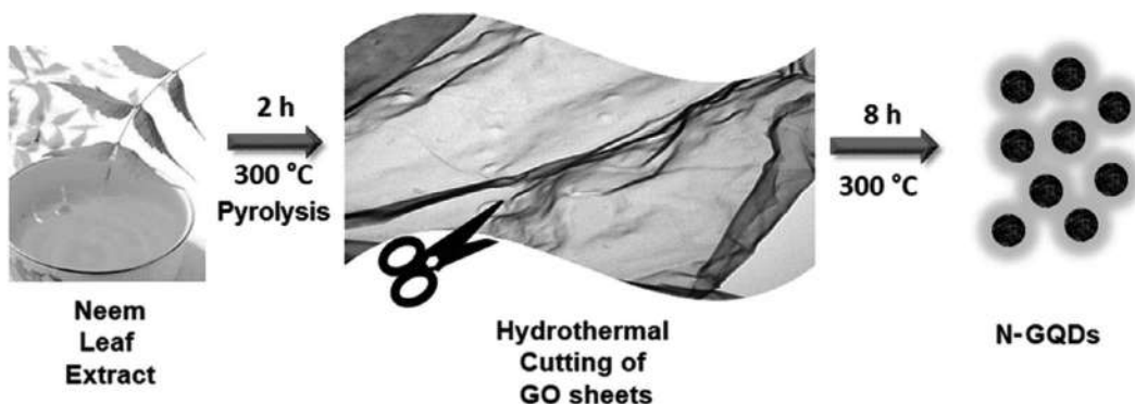
FIGURE 11.9 Schematic presentation for the preparation of the GQDs from the Neem leaf extract using hydrothermal method. (Reproduced with permission from Roy et al. 2014, RSC.)
