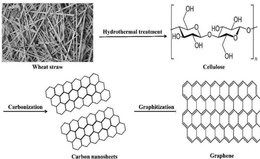
FIGURE 10.5 Schematic of the presented method to fabricate graphene from wheat straw. (Modified after Chen et al. (2016).)
