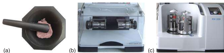
Figure 10.1 Laboratory instrumentation in mechanochemistry research: (a) mortar and pestle, (b) mixer ball mill, and (c) planetary ball mill.
