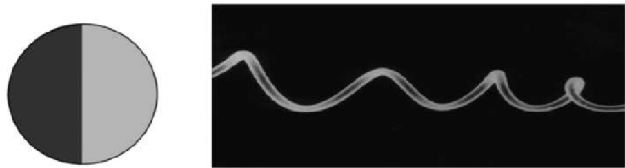
FIGURE 27.2 Cross-sectional view of side-by-side type of PLA bicomponent fiber and overview of the fiber with fine microcrimps.
