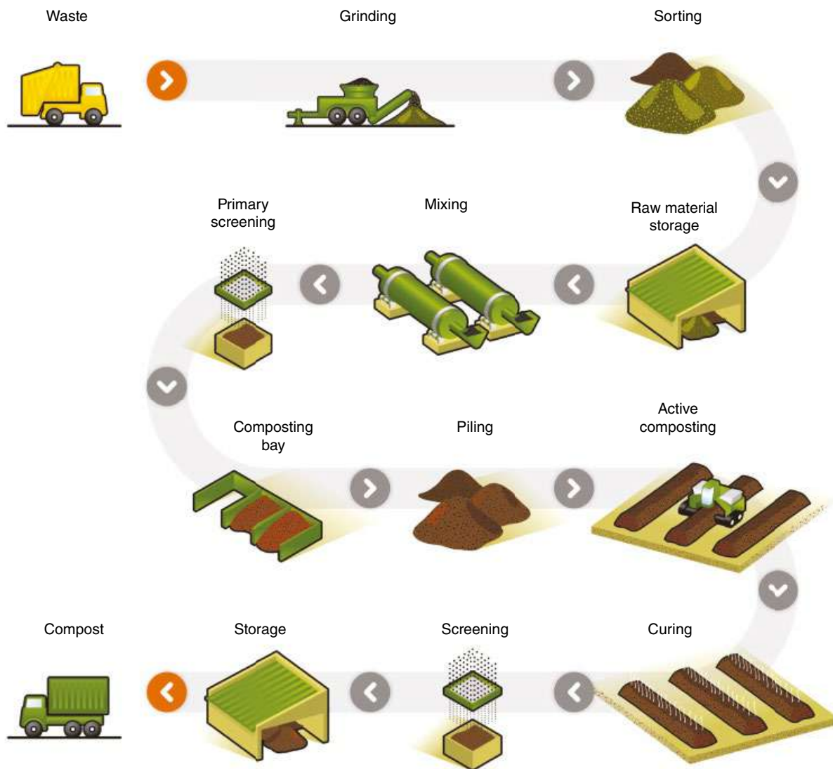
FIGURE 24.6 Steps of the composting process in an industrial facility. Source: Reproduced from Ref. [5].
