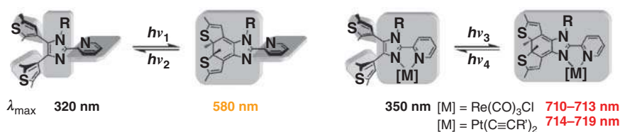
Figure 19.8 Photochromism and absorption maxima of diarylethene-containing 2-(2-pyridyl)imidazole ligands and their metal complexes. Source: Reproduced with the permission of American Chemical Society from Lee et al. [2].
