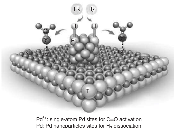
Figure 8.9 Schematic representation of bifunctional Pd 0 /Pd SA on TiO 2 . Source: Kuai et al. [65]. Springer Nature. CC BY 4.0.
