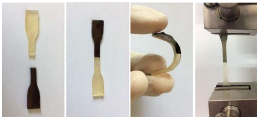
Figure 10.3 Elastomer self-healing based on shape memory effect [11].
