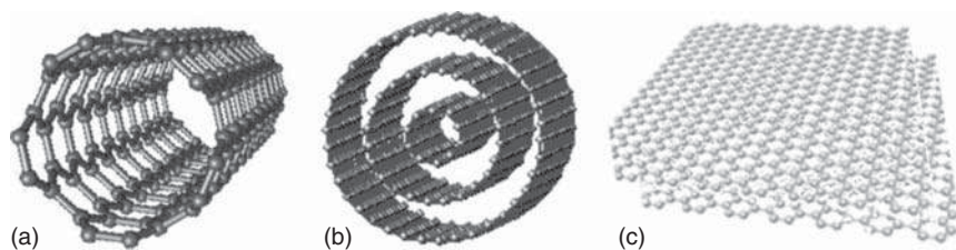
Figure 10.12 Conceptual diagram of (a) single-walled carbon nanotube (SWCNT), (b) multiwalled carbon nanotube (MWCNT) [58], and (c) graphene layer. Source: Reproduced from Geim and Novoselov [59]. © 2007, Springer Nature.
