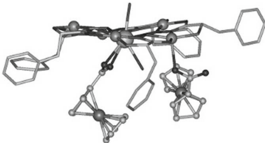
Fig. 22 Two ferrocenecarboxylate anions ( \text{FcC}^- ) are encapsulated in the hydrophobic cavity of (\text{La}^{\text{III}}[\text{15-MC}_{\text{Cu(II)N(L-pheHA)}-5}])^{3+} . One is bound monodentate to a copper ring metal with eclipsed cyclopentadienyl rings. The other is bound bidentate to lanthanum with staggered cyclopentadienyl rings. Unbound or Cu-coordinated solvent, nitrate, and hydrogens were removed for clarity. Reprinted with permission from John Wiley & Sons [113]
