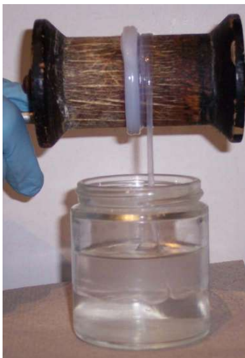
FIGURE 2.7 The “nylon rope trick”. The upper layer is 0.2 M sebacoyl chloride in hexane, and the lower layer is 0.5 M hexamethylene diamine in 0.5 M NaOH. Photo courtesy of J. Franek.
