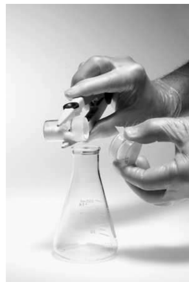
Figure 36-10 Quantitative transfer of solid sample. Note the use of tongs to hold the weighing bottle and a paper strip to hold the cap to avoid contact between glass and skin.
