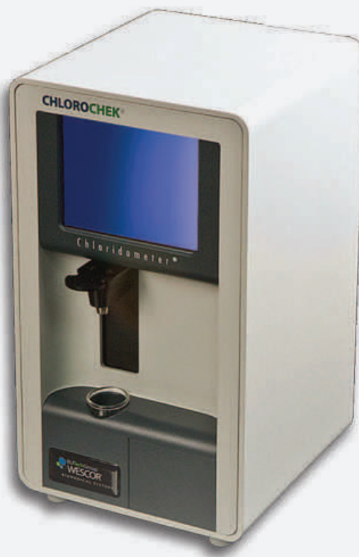
FIGURE 20F-2 A commercial digital chloridometer. This coulometric titrator is used to determine chloride ion in clinical samples and in food and environmental samples. The end point is detected by a pair of electrodes measuring solution conductance. (Courtesy of Wescor division of ELITech Group, 13-15 bis rue Jean Jaurès 92800 Puteaux, France.)
