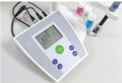
FIGURE 19-16 Photo of a typical benchtop pH meter. (korakot khayankarnavee/Alamy Stock Photo)
