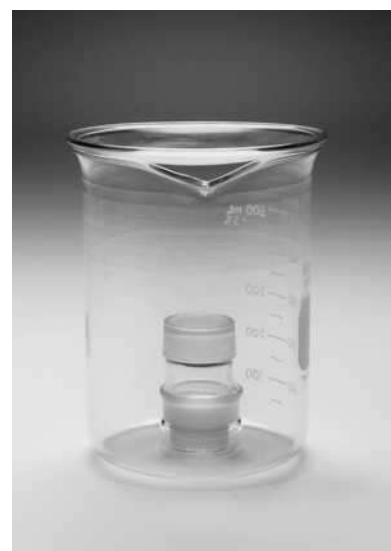
Figure 36-9 Arrangement for the drying of samples.
