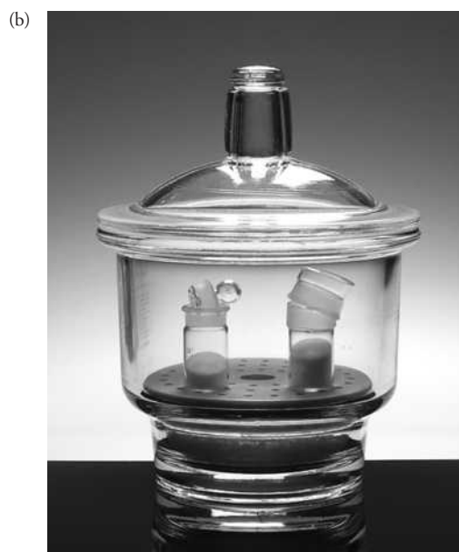
Figure 36-8 (a) Components of a typical desiccator. The base contains a chemical drying agent, which is usually covered with a wire screen and a porcelain plate with holes to accommodate weighing bottles or crucibles. (b) Photo of desiccator containing weighing bottles with dry solids.
