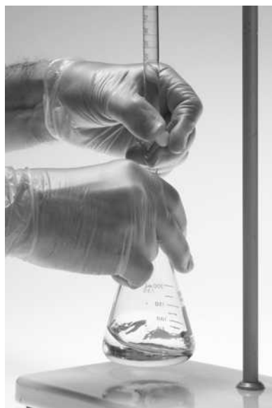
Figure 36-23 Recommended method for manipulating a buret stopcock.
