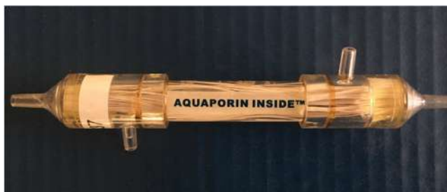
FIGURE 13.8 Photograph of Aquaporin Inside hollow fiber membrane module. Source: Reproduced from Ren, J., & McCutcheon, J. R. (2018). A new commercial biomimetic hollow fiber membrane for forward osmosis. Desalination, 442, 44–50.
