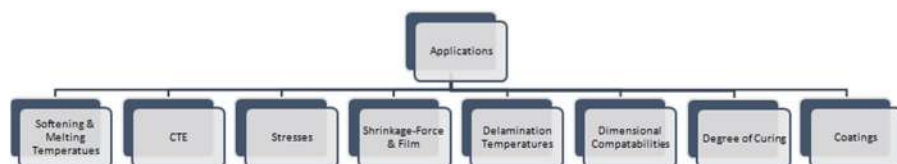
Figure 6.19 Applications of TMA in the area of polymers. TMA , Thermomechanical analysis.
