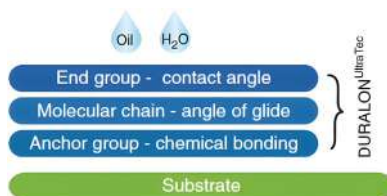
Figure 11.10 Modern mirrors' ultrareflective layer composition.
