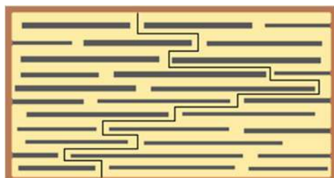
Figure 15.2 Tortuous path model of polymer nanocomposites.
