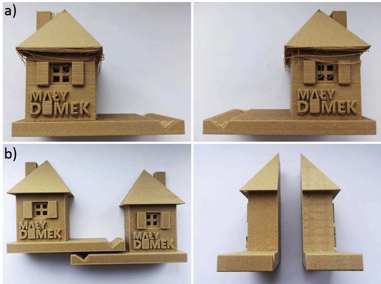
FIGURE 2.5 Printing of a telephone stand with a house-shaped support (A) in full, with an apparent problem of dangling threads during printing of the roof and writing on the wall, (B) in two parts, flat, which positively influenced the quality of printing. (Reprinted from Ref. [28]).
