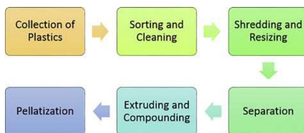
FIGURE 16.6 Process of waste conversion into pellets.
