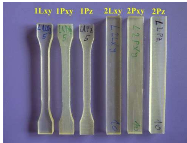
FIGURE 17.3 PVC test specimens made by SHL process [12]. Reprinted from Technical Gazette [12], Copyright (2011), with permission from Technical Gazette .
