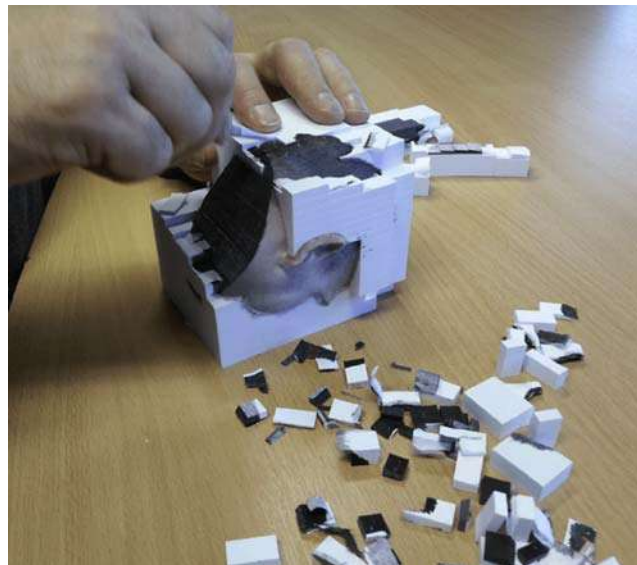
FIGURE 11.4 Process of removing support structure in the SDL [14]. (Source: courtesy of D. Herzberg).
