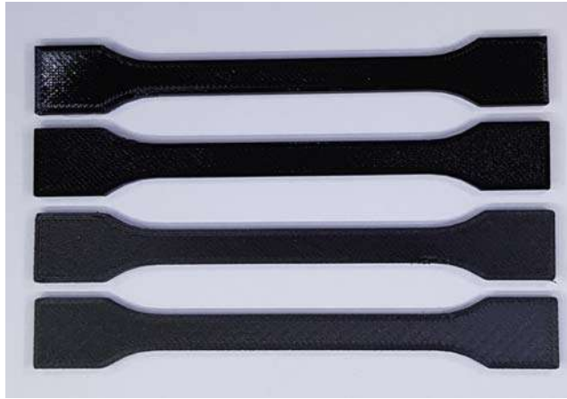
FIGURE 5.5 3D printed samples for testing the strength of materials.
