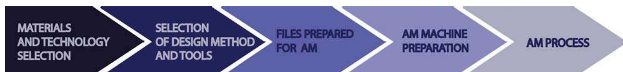
FIGURE 2.1 Flowchart of the model development and AM processes.
