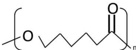
FIGURE 18.5 Chemical structure of PCL.
