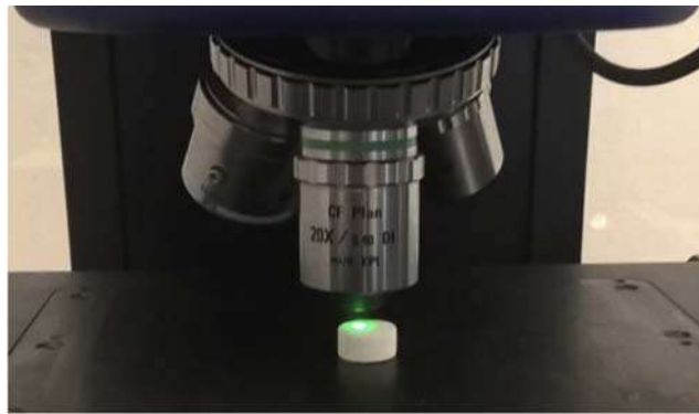
FIGURE 15.10 Model made of PA 2200 polyamide—during testing with the Taylor Hobson CCI optical profilometer.
