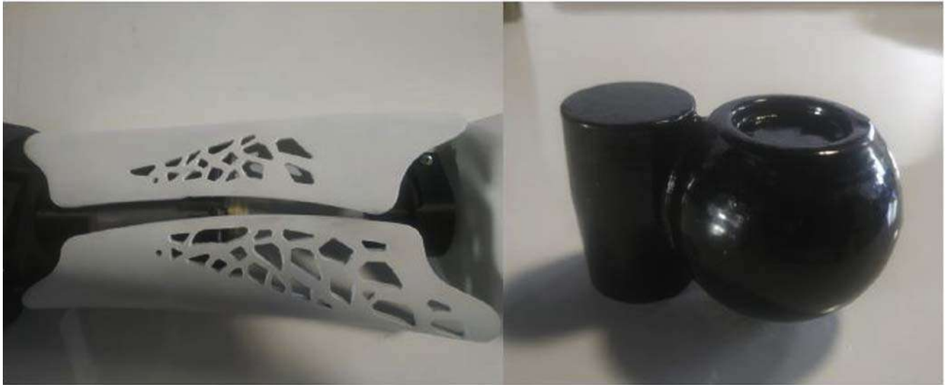
FIGURE 7.11 3D printout after mechanical ( left ) and chemical ( right ) processing.
