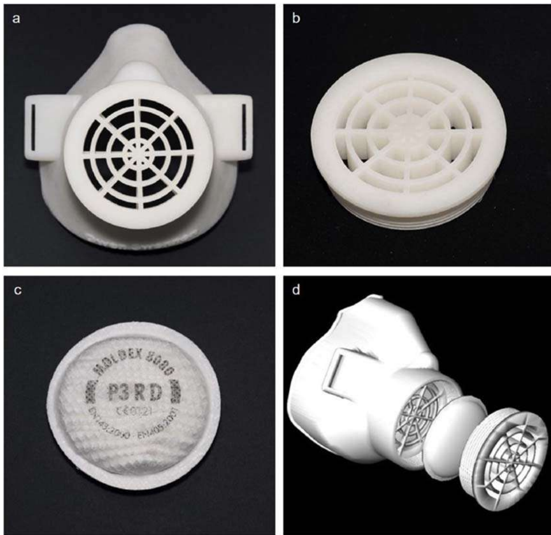
FIGURE 20.10 Protective mask printed and its components: (A) reusable 3D-printed face mask, (B) filter membrane support, (C) polypropylene (PP) non-woven melt-blown particle filter, and (D) 3D image of the prototype [51]. Reprinted from [51], Copyright (2020), with permission from Elsevier.
