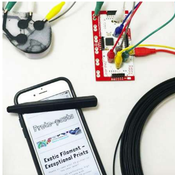
FIGURE 14.25 3D-printed objects made from conductive composite PLA printing filament. Image credits: ProtoPlant, makers of Proto-Pasta.
