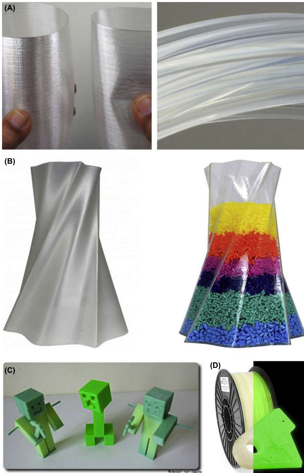
FIGURE 14.31 3D-printed objects from special 3D printing filaments: (A) translucent, (B) glass, (C) color changing, (D) glow in the dark. (A) From: Bendlay stiff and soft by Lay-Filaments & Kai Parthy; (B) Image credits: Smart Materials 3D printing; (C) Image credits: 3D FilaPrint; (D) Image credits: MatterHackers Inc.
