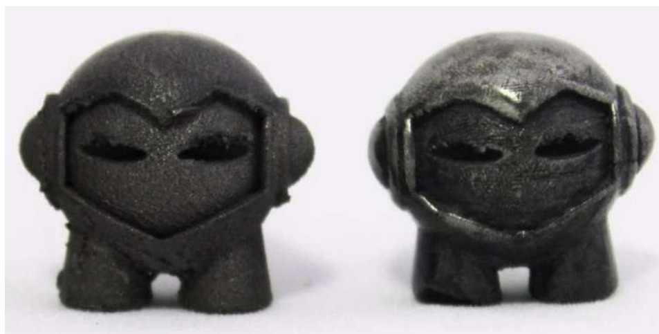
FIGURE 14.24 3D-printed object from steel-filled PLA printing filament. Image credits: ProtoPlant, makers of Proto-Pasta.
