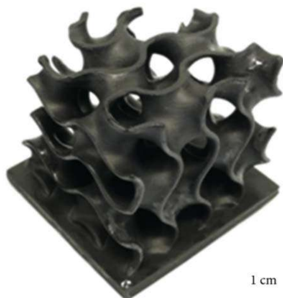
FIGURE 13.5 Graphene-reinforced nanocomposite gyroid scaffold for bone tissue engineering [54].
