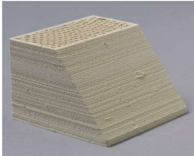
FIGURE 14.29 3D-printed object from sandstone filament. From: Bendlay stiff and soft by Lay-Filaments & Kai Parthy .
