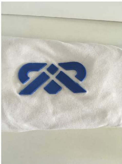
FIGURE 14.18 3D-printed object from TPU and TPU printed on the textile material. (A) Image credits: AMFG – amfg.ai . (B) Image credits: UL NTF.
