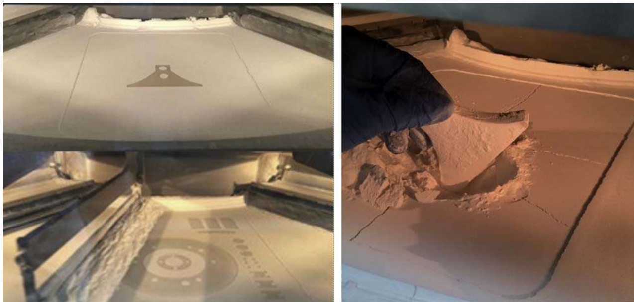
FIGURE 15.1 Selective laser sintering printing platform (Formiga P100 machine); material—polyamide PA 2200.
