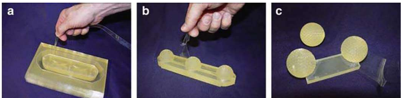
FIGURE 11.6 The process of separating excess PVC material [3]. Reprinted from [3], Sheet lamination processes , Copyright (2010), with permission from Springer.
