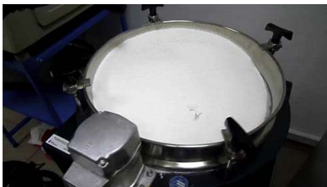
FIGURE 15.3 The process of screening and mixing the used and fresh powder using a vibrating agitator.
