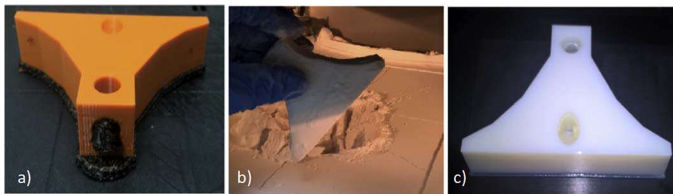
FIGURE 15.4 Printing of models from materials in the form of: (A) solid, (B) powder, (C) liquid (resin).
