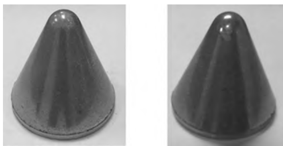
Fig. 13.24: A pressed (left) and sintered (right) PTFE/W/Cu/Pb SC liner.
