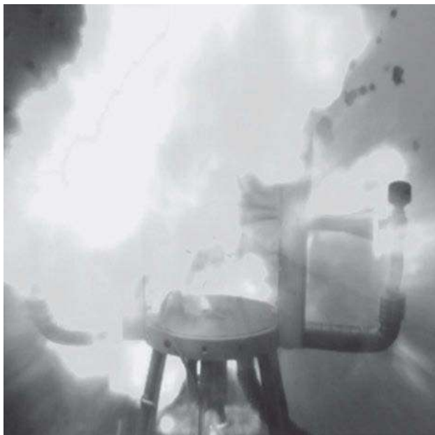
Fig. 9.23: Explosion of bis(trinitroethyl)-1,2,4,5-tetrazine-3,6-diamine (BTAT) in Koenen test.
