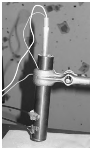
Fig. 7.17: Typical set-up for a simple determination of the detonation velocity using the optical fiber method.
