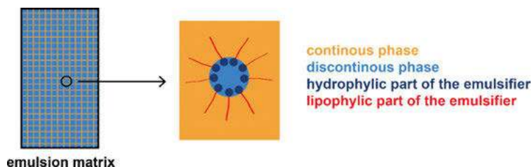
Fig. 13.18: Arrangement of the emulsifier in a water-in-oil emulsion.
