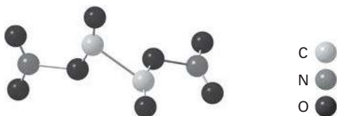
Fig. 4.8: Transition state structure for the simultaneous dissociation of \text{O}_2\text{N}-\text{O}_2\text{C}-\text{CO}_2-\text{NO}_2 into \text{CO}_2 and \text{NO}_2 at CBS-4M level of theory (NIMAG = 1, \nu_1 = -817 \text{ cm}^{-1} , d(\text{C}-\text{C}) = 2.33 \text{ \AA} , d(\text{O}-\text{NO}_2) = 1.91 \text{ \AA} ).
