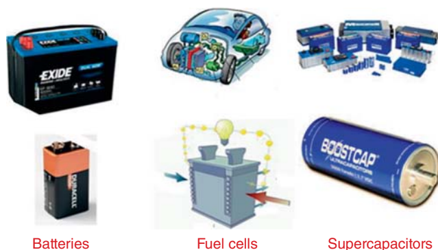
Figure 8.4 Types of electrochemical energy storage devices. Source: Maxwell Technologies, Inc./Wikimedia commons/CC by SA 3.0.
