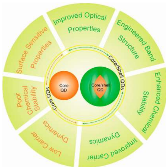
Figure 21.1 Properties of bare QDs versus core–shell QDs.
