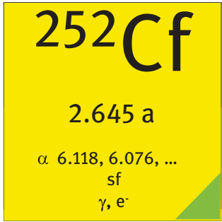
Fig. 10.19: Transformation properties of the spontaneous fission-based neutron source ^{252}\text{Cf} .
