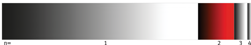
Fig. 1.7: Schematic energy scale of electron binding energy in proportions according to eq. (1.1). Starting with the energy level for n = 1 , any higher energy level is fractionated due to the E_{B(e)}(n = 1) value as 1/4 , 1/9 , 1/16 , 1/25 etc. for E_{B(e)}(n = 2) , E_{B(e)}(n = 3) , E_{B(e)}(n = 4) , E_{B(e)}(n = 5) , respectively.
