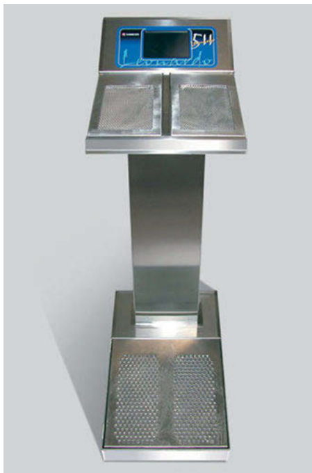
Fig. 1.31: A typical hand-and-foot contamination meter (Comecer S.p.A., Castel Bolognese, Italy). Four plastic scintillators (two for the hands, two for the feet) are read by PMTs and the readout is shown in real-time on the LCD display, after calibration in \text{Bq/m}^2 for several types of radionuclides (user-selectable). (From http://www.centroditaratura.it/servizi-taratura/strumenti/mani-piedi-vesti/ – last access on June 9, 2012).
