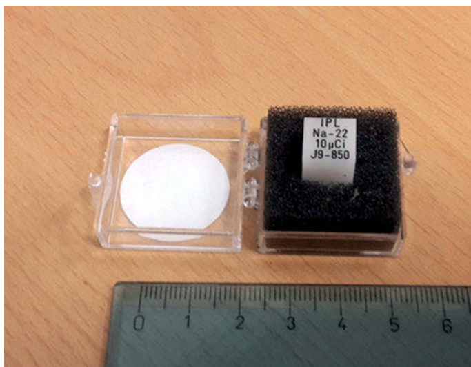
Fig. 1.22: Example of a sealed point Na-22 source for calibration of PET scanners.
