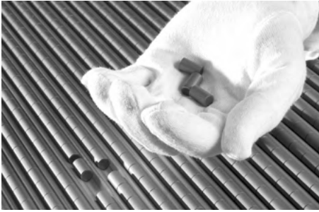
Fig. 10.4: Fuel pellets, FBFC Romans (© AREVA, Geoffray Yann).
