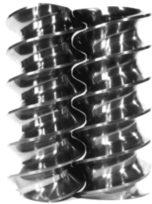
Fig. 1.13 Screws of a Twin Screw extruder [clextal.com]
