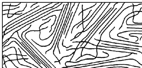
Fig. 7.8 Morphological structure of the semi-crystalline polymer [13]
