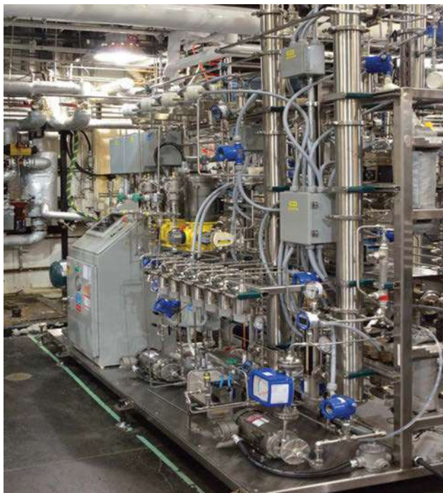
Figure 2.2: The demonstration unit for wastewater purification, built by Forward Water Technologies in Mississauga, Canada.
