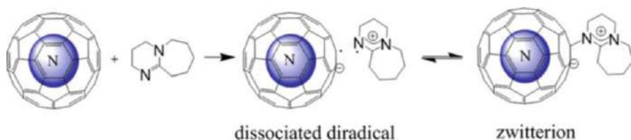
Fig. 11 Direct interactions between DBU and ENF, which form a dissociated diradical and zwitterion
