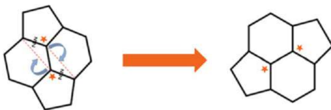
Fig. 3 Illustration of a Stone-Wales transformation
