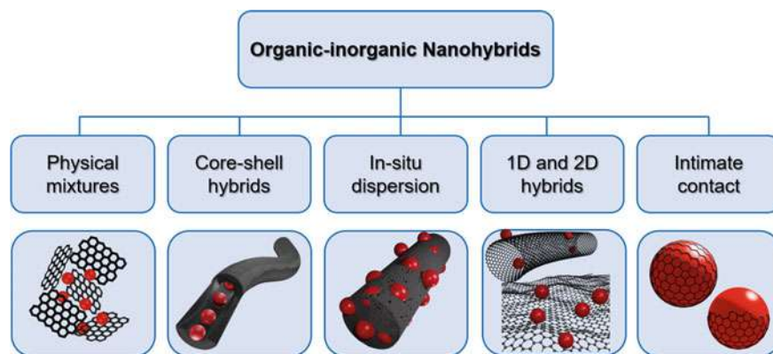
Fig. 5 Classification of organic (black)–inorganic (red) hybrid based on their interface
