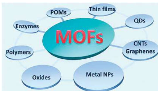
FIG. 1.3 The scheme for the composites of MOFs and functional materials. (Reproduced with permission from Q. Zhu, Q. Xu, Metal-organic framework composites . Chem. Soc. Rev. 44 (2014) 5468–5512. Copyright 2014 Royal Society of Chemistry.)
