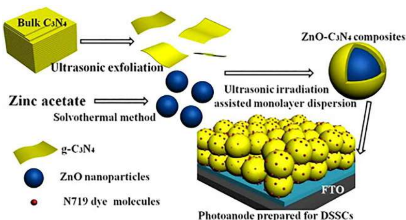
Figure 6.18 Fabrication mechanism of a g-C 3 N 4 /ZnO photoanode in DSSCs. Reproduced from ref. 91 with permission from Elsevier, Copyright 2015.
