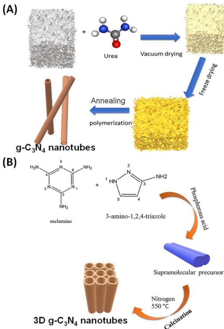
Figure 1.3 (A) The formation mechanism of gCN nanotubes through a melamine sponge. 79 (B) The mechanism of the as-synthesized 3D gCN cage consisting of nanotubes. 80
