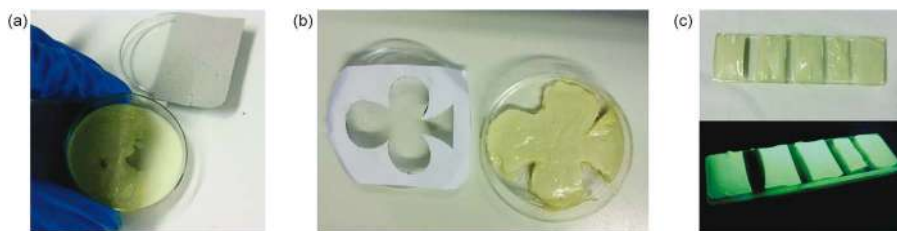
Figure 5.5 Control of photopolymerization for gel synthesis in a spatial way: (a) self-standing half-circle, (b) self-standing club shape and (c) photopatterned stripes on glass. Reproduced from ref. 99 with permission from the Royal Society of Chemistry.
