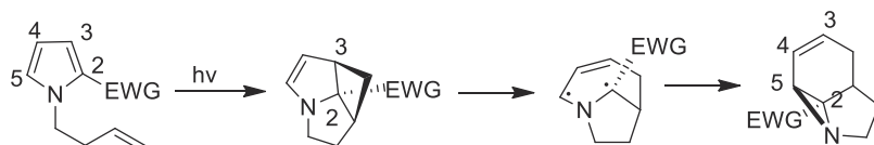
SCHEME 1.9 Mechanism of the reaction.
