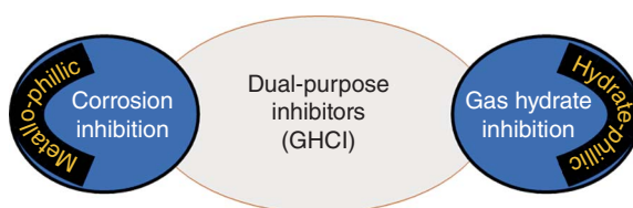
Figure 8.4 Proposed functionality of dual-purpose corrosion inhibitor.
