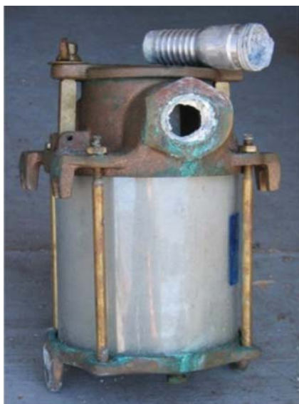
Figure 13.3 Galvanic corrosion on aluminum hose barb. Source: Popoola et al. [15]/Springer Nature.
