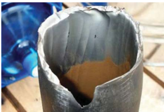
Figure 13.5 SCC has affected an oil and gas pipeline. Source: Popoola et al. [15]/Springer Nature.
