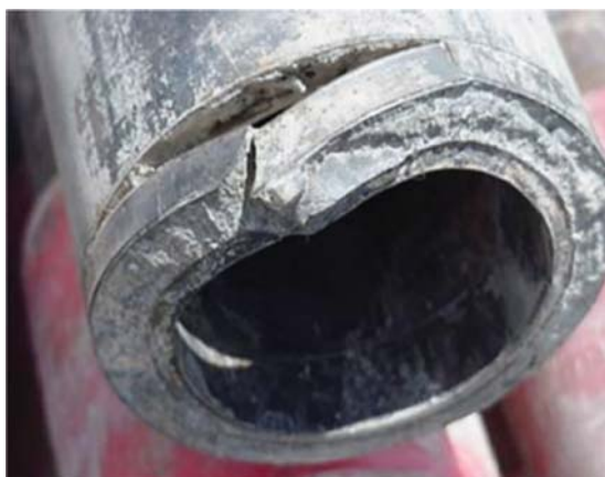
Figure 13.6 Oil and gas pipeline in sour condition. Source: Popoola et al. [15]/Springer Nature.
