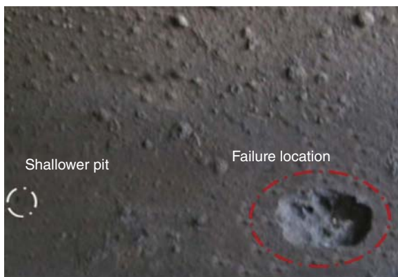
Figure 13.4 Pitting corrosion on the internal surface of the wet gas pipeline. Source: Mansoori et al. [16]/Elsevier.
