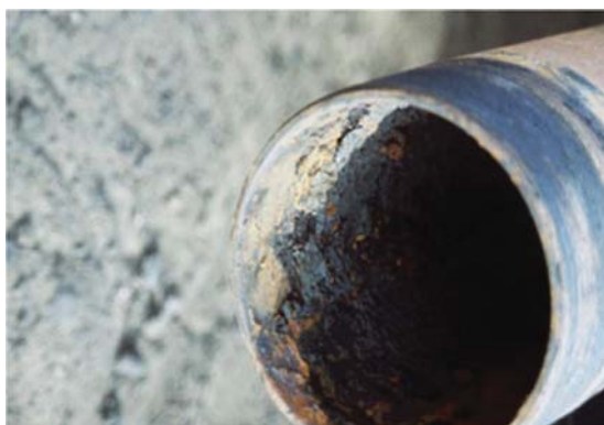
Figure 13.8 Corrosion due to oxygen. Source: Popoola et al. [15]/Springer Nature.
