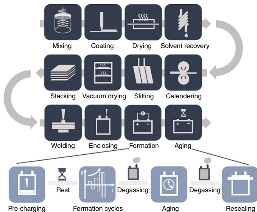
Figure 4.4 EV power battery production process. Source: Liu et al. [12] / with permission of Elsevier.
