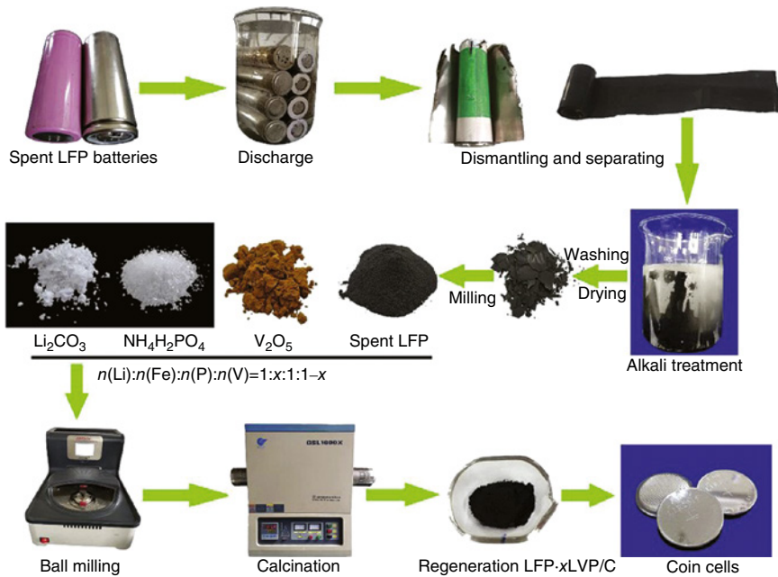
Figure 2.16 Recovery process of spent \text{LiFePO}_4 . Source: [57] Xu, B. et al., (2019), Elsevier.
