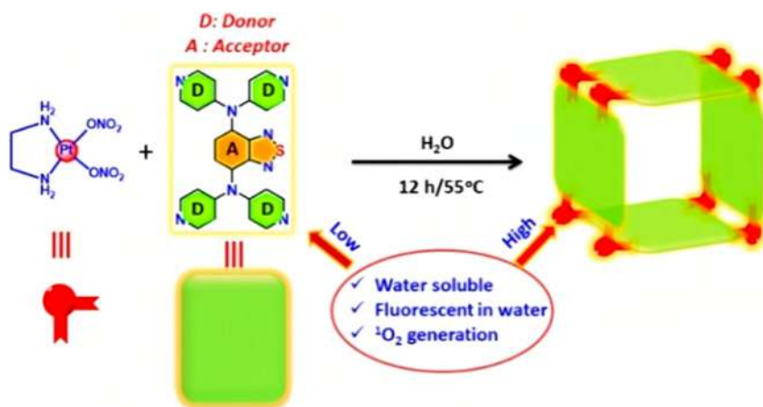
FIGURE 12.16 Benzothiadiazole-based tetrapyrrolyl ligand and Pt metallosupramolecular.
