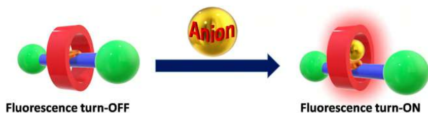
FIGURE 15.11 Cartoon showing the function of rotaxne-based turn-ON fluorescent sensor.
