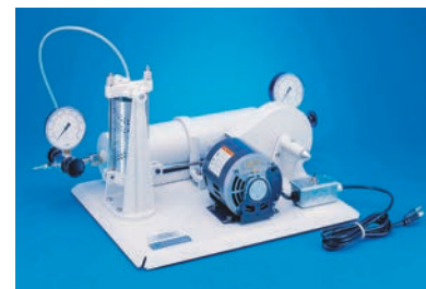
The Parr hydrogenation apparatus shakes the reaction vessel (containing the alkene and the solid catalyst) while a pressurized cylinder supplies hydrogen.
