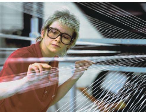
Production of continuous-filament nylon tire cord.
