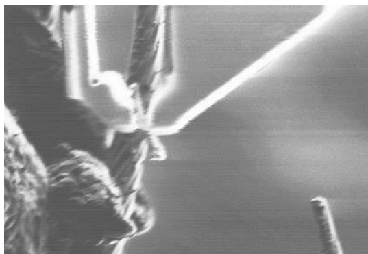
Figure 13.8. Manipulation of the biological microobjects by using \text{Ti}_2\text{NiCu/Pt} composite nanotweezers with SME in the vacuum chamber of the scanning electron microscope: processing of the selected submicron bioobject by FIB.
