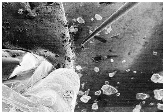
Figure 13.6. Manipulation of the biological micro-objects by \text{Ti}_2\text{NiCu/Pt} composite nanotweezers with SME in the vacuum chamber of the scanning electron microscope: comparison of the size of the composite nanotweezers with the leg-size of the insect ( Culex pipiens ).
