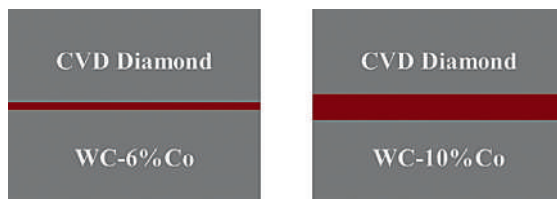
Figure 14.2. Thermal stress in diamond films increases with an increase in cobalt content. The red line represents the thermal stress generated at the diamond–tungsten carbide interface.
