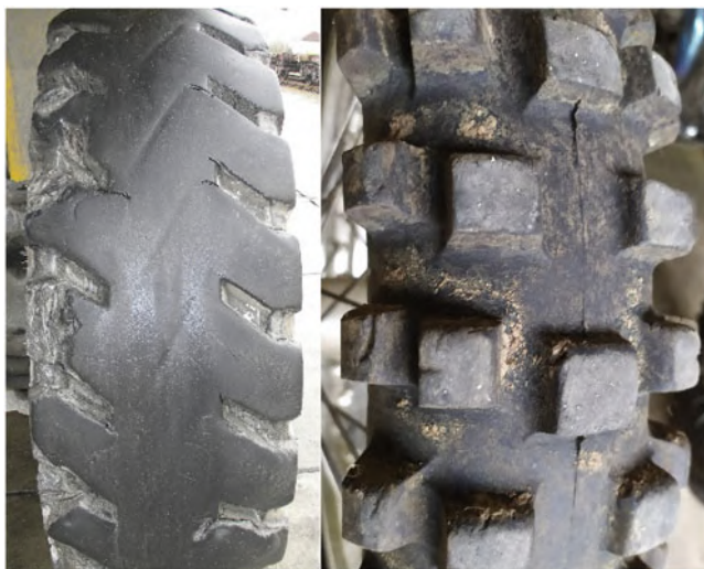
Fig. 2 Photographs of the worn tire treads illustrating the wear mechanism
