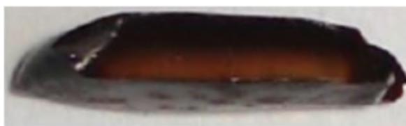
Fig. 16 Cross-section of HNBR specimen, aged at 160°C for 72 h
