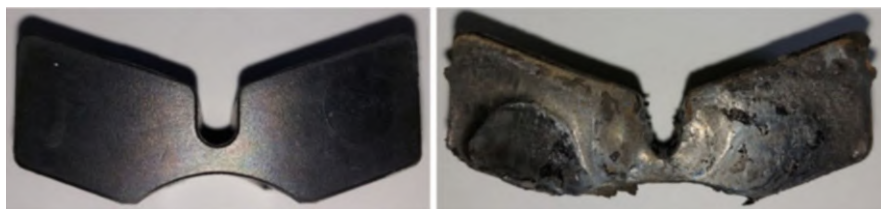
Fig. 1 Unused (left) and thermally degraded (right) rubber segment (Bonatrans Group a.s., Czech Republic)
