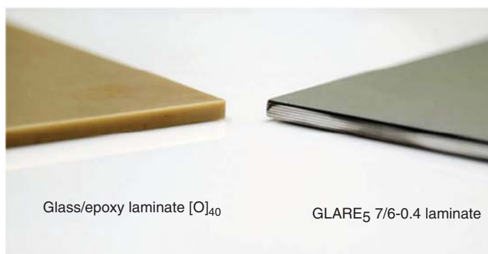
Figure 4.1 Photograph of glass/epoxy and GLARE laminates. Source: Park et al. [32].
