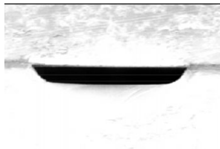
Figure 7.3 Cross-sectional view from a scanning microscope of a canal 20 \mu\text{m} high and 100 \mu\text{m} wide, etched in glass and covered with a silicon wafer (the system was microfabricated by ESIEE, and the photo taken at the Laboratory de Physique des Solides at ESPCI).
