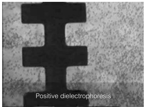
Figure 4.12 (Left) Schematic distribution of charges induced by a neutral particle submitted to an electric field in a vacuum. (Right) an experiment carried out in a microsystem showing that positive dielectrophoresis leads to an accumulation of particles in the regions where the field is at a maximum. Here, that maximum lies around the electrodes.
