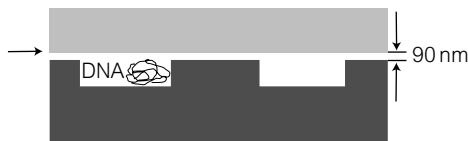
Figure 4.11 Basis of this experiment of Craighead et al. (1999). DNA molecules migrate from left to right in a system consisting of 1-μm wide cavities and 90-nm wide restrictions. The molecule must lose entropy to get through these restrictions; this system is thus known as an ‘entropic trap.’
