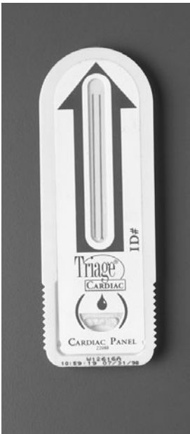
Figure 11 Biosite chip. A droplet of blood is placed in an opening on the chip. This drop is pulled towards the microfilter and the microseparator (in the direction of the arrow) by capillarity. The results of the analysis are given after data is analysed on a microcomputer. In just 15 min, this diagnostic can determine whether or not a heart attack has taken place.
