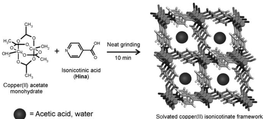
FIGURE 9.16 Mechanochemical synthesis of a porous MOF by neat grinding. 22
