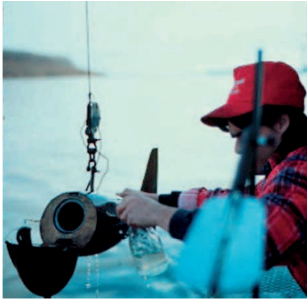
Figure 1 Suspended sediment sampling on the Mississippi River.
