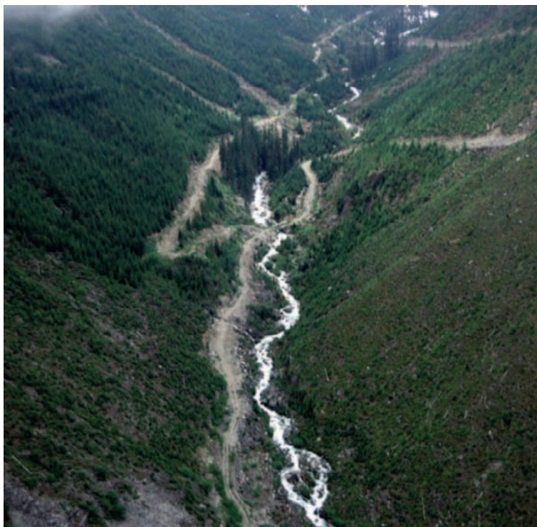
Figure 9 Road construction on moderately steep slopes adjacent to a stream channel, with no buffer strip of undisturbed vegetation in south western British Columbia, Canada, 1999. Photograph by Michael Feller.
