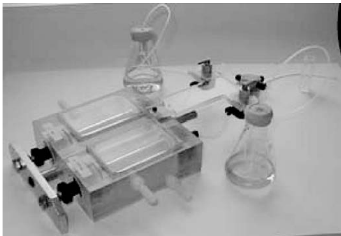
Figure 5.6 This home-made rapid mixer houses two 10 ml gas-tight Hamilton syringes that are encased in a block of plexiglass equipped for a temperature-controlled water bath. Three-way taps allow for solution uptake into the syringes and then equal volume delivery into a small mixing chamber before delivery into the cuvette.
