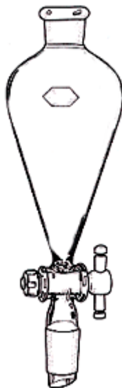
A standard laboratory separatory funnel.
