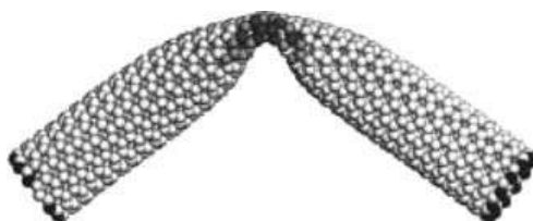
FIGURE 1.9 MD simulation of a large-amplitude transverse deformation of a carbon nanotube, apparently beyond the elastic limit. In fact, the tube snaps back once the computer-generated force is removed, and there is no plastic deformation or permanent damage. (From Yakobson, B. I., Appl. Phys. Lett. 72 , 918–920 (1998), with permission.)
