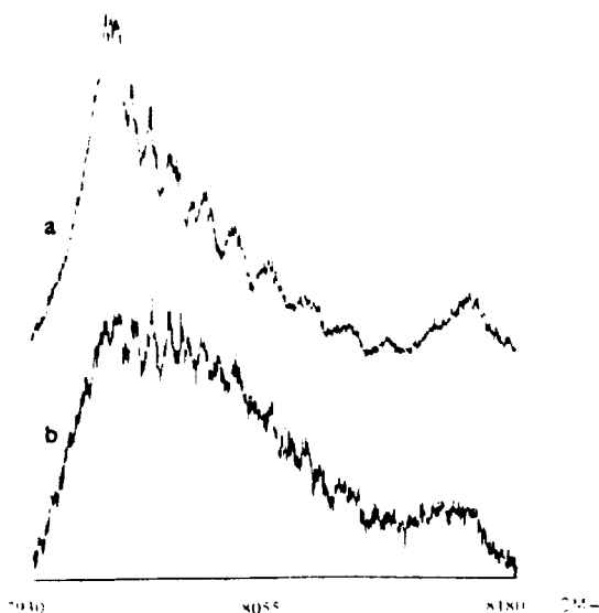
Fig. 4. Details of high-resolution spectra in the IR. (a) Emission: resolution = 0.25 \text{cm}^{-1} ; recording time: 2 h 20 min; same conditions of the reaction as in fig. 2. (b) Absorption: resolution = 0.25 \text{cm}^{-1} ; recording time: 1 h; same conditions of the cell as in fig. 3.
